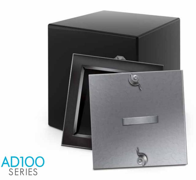
EXCELAIR Access Doors/Panels (AD 100 Series) are used in GI/MS/SS Air Ducts to access the Fire Dampers, VCDs, Filters etc. for servicing. They are manufactured as per standardized or customized needs. Generally manufactured in 0.7mm thick Galvanized Iron Sheet matching the quality of ASTM A653M – LFQ (supersedes ASTM A525/A527) unoiled, chromated, regular spangle zinc coating Z27/G90/G275 (275 gms/sqm).
